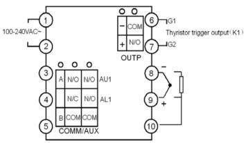
parameter bAud = 2, it can be used for AU1 or AL1 alarm output. If L1, L2, L4, G, K1, W1 or W2 is installed, it can be the auxiliary output in bidirectional (heating/refrigerating) control (Auxiliary output doesn't support analog current output); if I2 is installed and bAud = 1, then it can input on-off signal to switch SV1 and SV2 (AI-518) or switching the program status RUN / Stop (AI-518P) by connecting a switch between terminals number 3 and 5.
