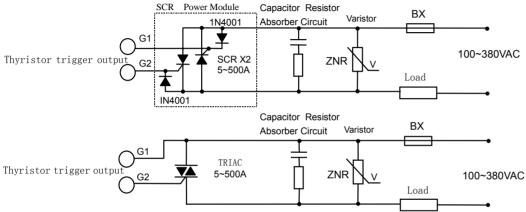
Note 1: According to the voltage and current of load, choose suitable varistor to protect the thyristor. A resistor-capacitor circuit (RC circuit) is needed for inductance load or phase-shift trigger output.
