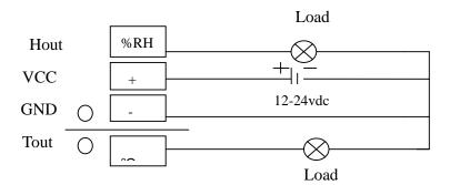
**E.g** . It is assumed it is temperature and humidity transmitter, 4-20mA output, connection as follows:
